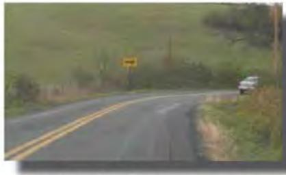
*One direction Large Arrow Sign placed within curve.*
