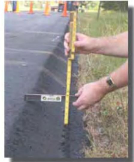
*Technique for measuring height and depth of drop-offs.*
