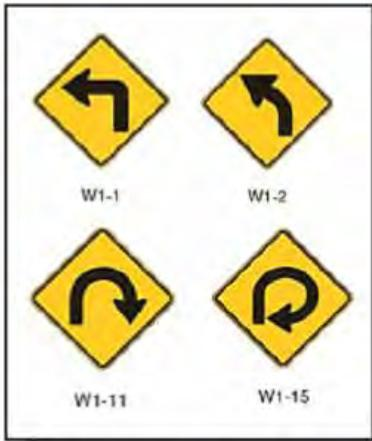
*The MUTCD prescribes Horizontal Alignment Signs for advanced warning of a single curve section.*
