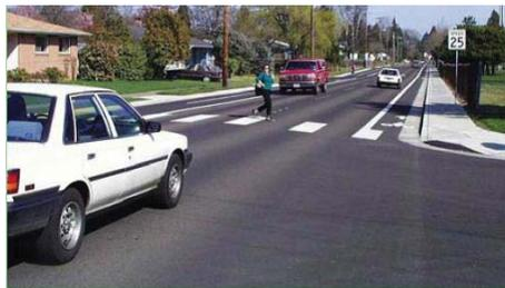
On multi-lane roadways, marked crosswalks without a raised median are NOT recommended on roadways with greater than 12,000 ADT (see example below).
