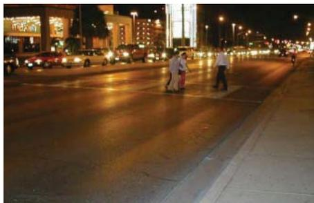
On multi-lane roadways with an ADT of greater than 15,000 ADT, marked crosswalks even with a raised median are NOT recom-
